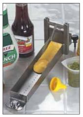
Determine the consistency and flow rate of viscous materials.
